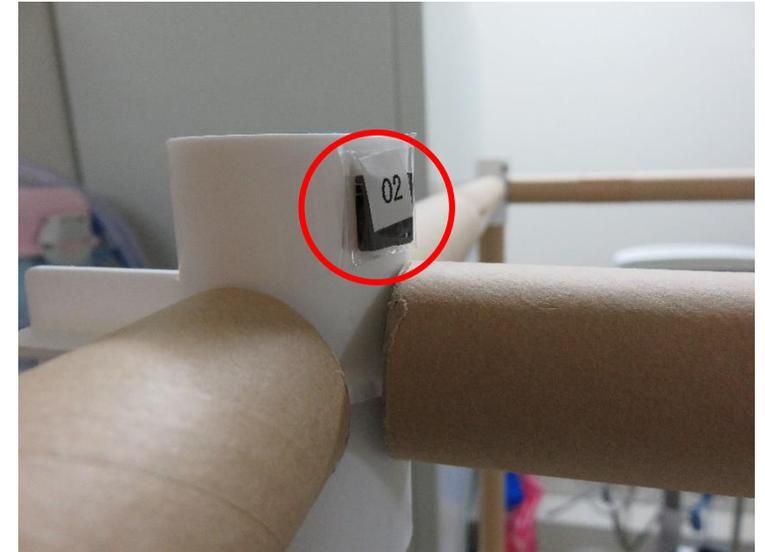
Small OSL dosimeters were attached to the connection parts of the paper pipes, facing the direction of the radiation source.
